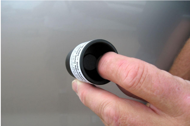
1. Insert the RMS-Plus™ delay element to be drilled into the well in the Delay Drilling Adapter (DDA).
