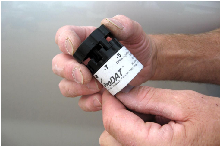
2. Set the ProDAT for the desired number of seconds to be removed from the delay (note the AeroTech delay equivalency on the DDA label).
