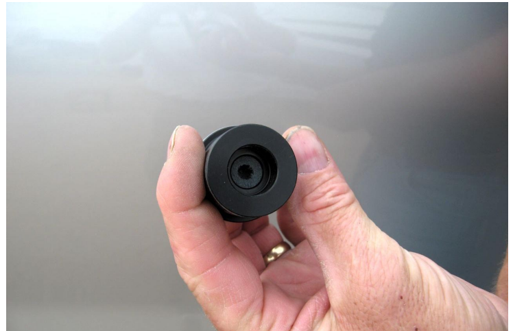
5. Remove the DDA from the Pro-DAT and verify that the delay element has been drilled to the depth desired. Destroy the "tailings" from the drilling process by igniting electrically in a safe location.
