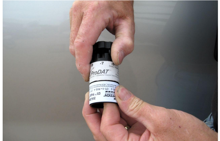
4. Continue holding the delay element in the DDA and turn the Pro-DAT against the DDA until the flange on the DDA "bottoms out" against the Pro-DAT.
