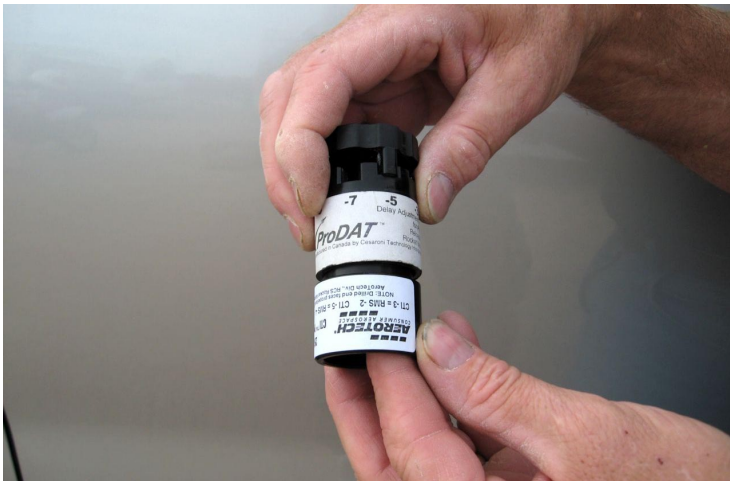
3. Holding the delay element firmly in the well of the DDA, insert the smaller-diameter portion of the DDA into the drilling well of the Pro-DAT.
