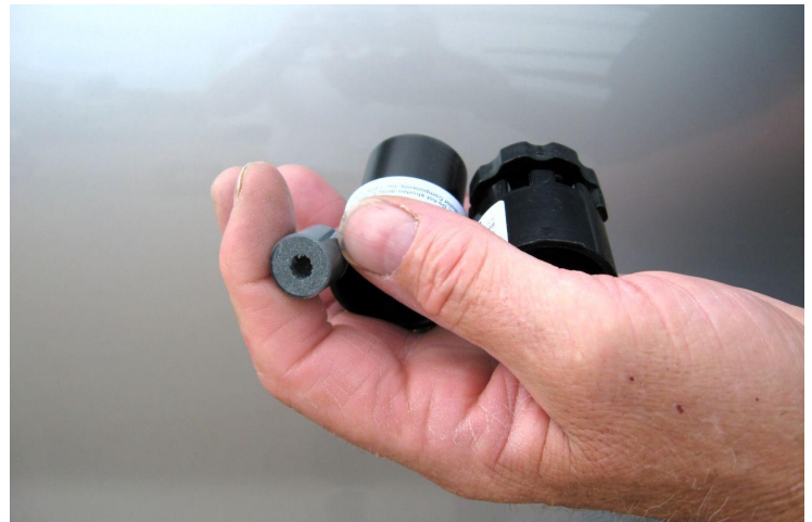
6. Remove the delay element from the DDA and install in your motor per the AeroTech RMS™ reload kit instructions, with the drilled end facing the propellant grain(s).
