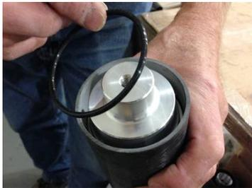
1.3 Raise the motor assembly into a vertical position and ensure that the bulkhead and liner assembly is fully seated in the case and against the nozzle. The larger diameter of the bulkhead should now be flush with the end of the case. Place the (thicker) forward O-ring into the space between the smoke bulkhead and the case. **CAUTION: Do not** apply any grease to the forward O-ring and do not allow any oil or grease to contact the interior abraded end of the case.
