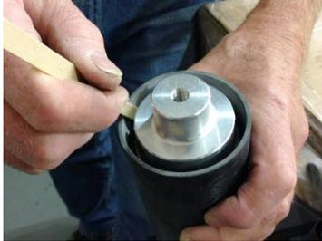
1.4 Using a stir stick or a flat blade screwdriver, push the forward O-ring completely into the groove between the smoke bulkhead and the case. **CAUTION: Do not** allow any oil or grease to contact the interior abraded end of the case.
