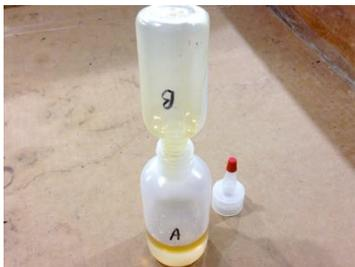
2.1 Remove the screw-on caps of the supplied epoxy bottles and dispense the contents of the smaller hardener bottle into the larger resin bottle. Allow the hardener bottle to drain into the resin bottle for 30 seconds.
