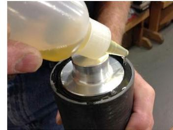
2.3 Replace the screw-on cap of the larger bottle and dispense enough of the mixed epoxy into the space between the smoke bulkhead and the case to fill it completely. Secure the completed motor assembly to a stable, solid object (such as a table leg) in a vertical position and allow it to cure for at least 16-24 hours prior to use.
