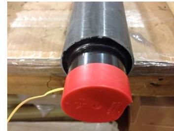
3.3 Insert the black-coated end of the igniter into the nozzle opening and push it completely into the motor core, until the coated end is touching the smoke element in the motor bulkhead.
