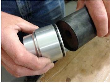
1.2 Insert the larger end of the smoke bulkhead with the pre-greased O-ring into the open end of the liner. Use a twisting motion to ensure the bulkhead flange is seated completely against the liner.
