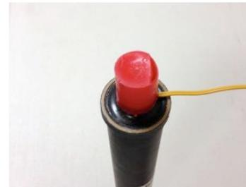
3.4 Using a hobby knife or scissors, cut a corner off the end of the nozzle cap (if supplied) to produce a vent hole in the cap about 1/16"-1/8" wide.
