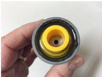
2.2 Place the ejection charge baffle washer into the ejection charge well of the motor bulkhead.
