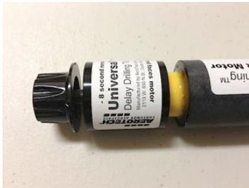
1.3 Place the open end of the tool over the motor bulkhead, hold the tool and motor firmly against each other and turn the drill knob several times clockwise until the drill knob sits flush against the drill tool body.
