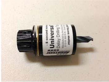
1.2 **Optional:** Place the washer between the drill knob and the tool if you want to remove 2 seconds less than the value printed on the tool (i.e., - 2 or - 6 seconds removal). **CAUTION: Do not** shorten the time delay to a value of less than 6 seconds.
