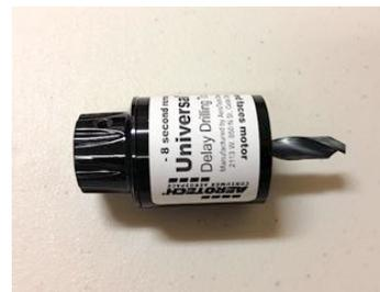
**1.1 WARNING:** Do not smoke and ensure that there are no open flames or heat sources nearby when setting the time delay. Assemble the AeroTech Universal delay drilling tool with the desired amount of delay time removal (i.e., the - 4 or - 8 seconds removal marked on the tool label) facing the exposed drill bit and motor bulkhead.
