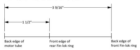
Use the LOCATION GUIDE above to make pencil marks along the motor tube line for location of the FIN-LOK rings per STEP 3. The new marks will move the motor tube rearward so that it is flush with the end of the body tube.
